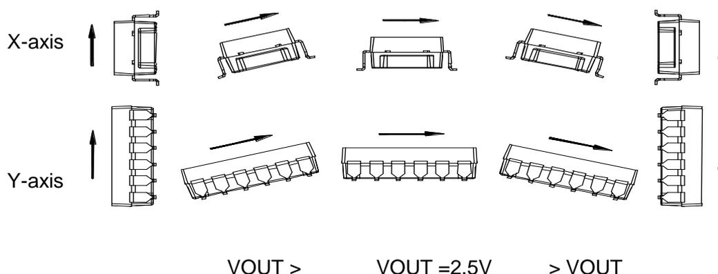
Figure 4. The measuring directions of the SCA1000
