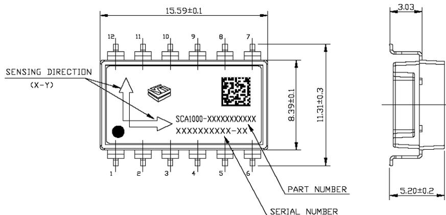
Figure 11. Mechanical dimensions of the SCA1000 (Dimensions in mm)
