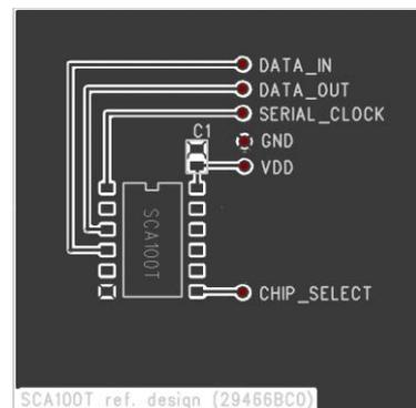
Figure 9. SPI connection example
