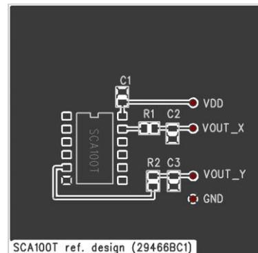
Figure 8. Analog connection and layout example
