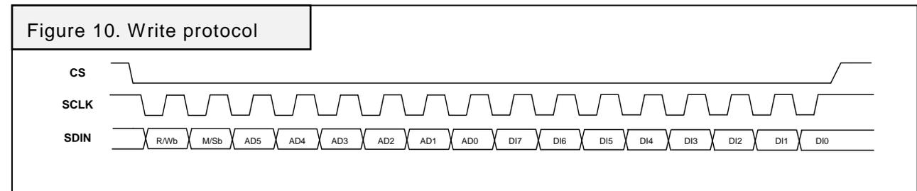
The SPI Write command is performed with 16 clock pulses. The multiple byte write command is performed adding blocks of 8 clock pulses at the previous one.
