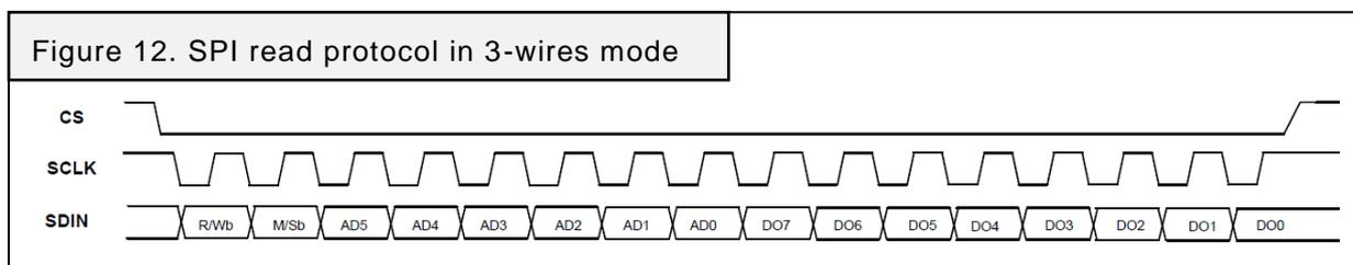
The SPI read command is performed with 16 clock pulses:
