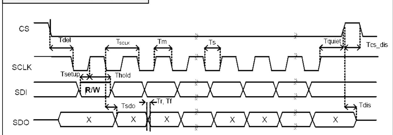
The device SPI is a bus slave. The SPI allows to write and read the registers of the device. The serial interface interacts with the outside world with 4 wires: CS, SCLK, SDIN and SDOUT.
